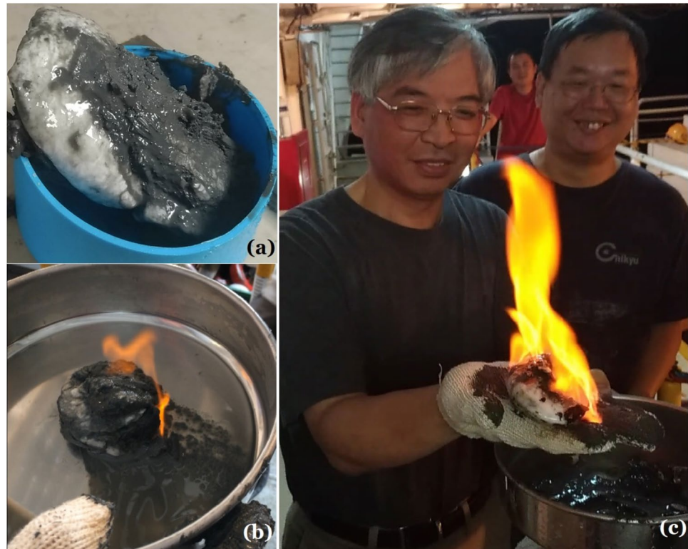
Fig. 3 a The gas hydrate sample collected at core site MD18-3542, and b the sample collected at core site MD18-3543. c The burning gas hydrate obtained at core site MD18-3542. The person who holds the burning gas hydrate is Prof. Shu-Kun Hsu, and next to him is Prof. Chih-Chieh Su
